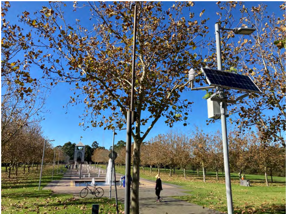
Figure 33. A solar-powered weather station deployed on a ridgeline and major thoroughfare within Bicentennial Park. Image credit: UTS
