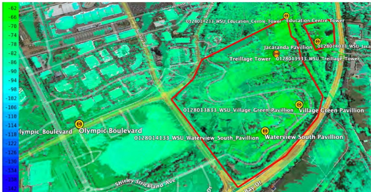
Figure 18. The Radio Frequency map used to identify optimal locations for LoRaWAN gateway deployment.
